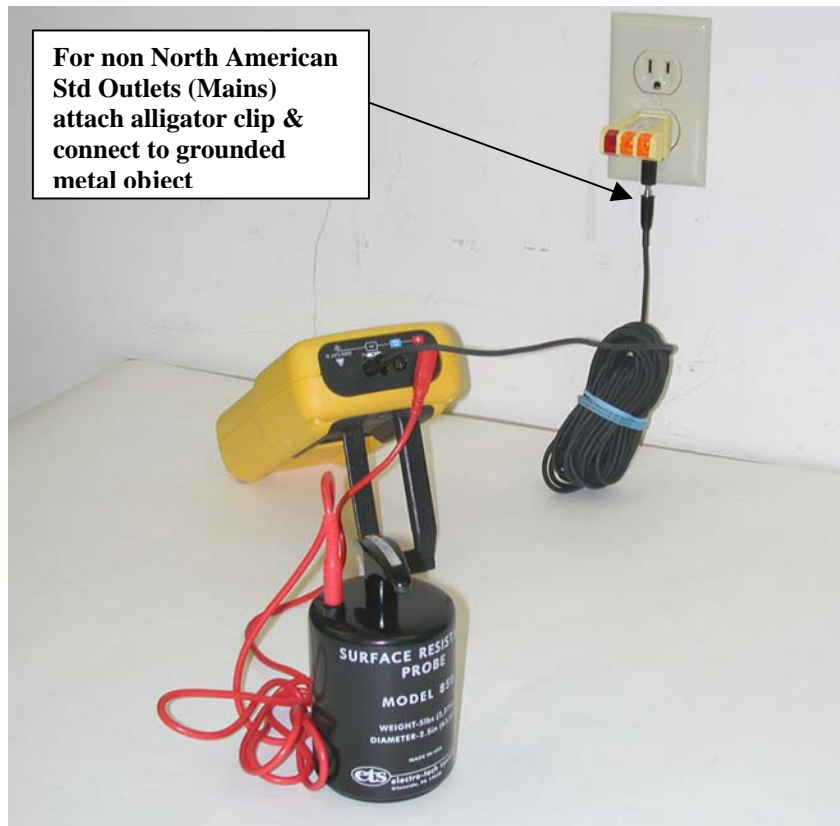
Figure 5.2-1: Typical RTG meter/probe hook-up
