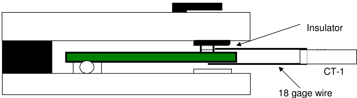
Figure 6.0-1: Calibration set up to measure ESD pulse
