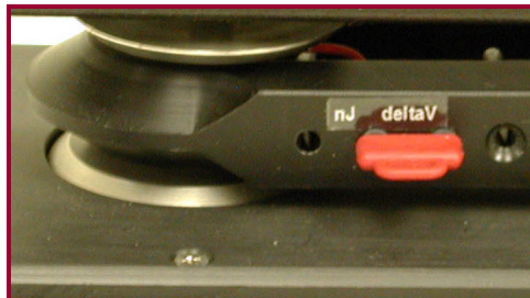
Figure: 5.0-3 Capacitive Sensor conversion from energy to voltage
