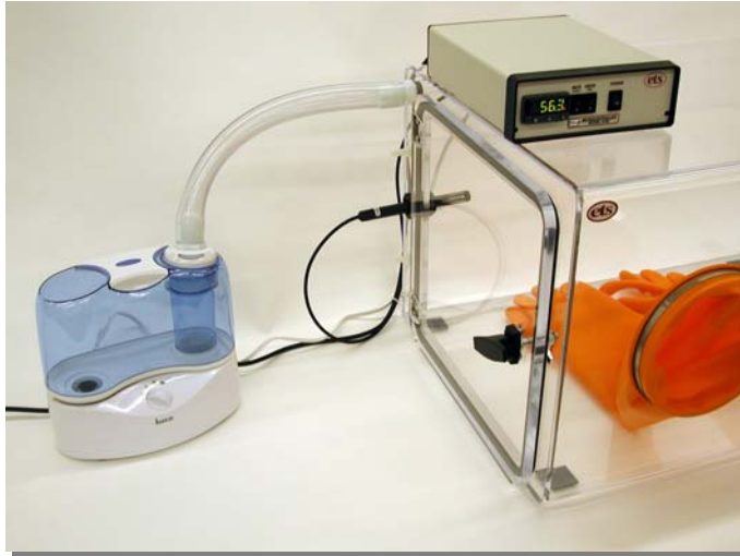
Figure 1.2-1: Package C Humidification System
