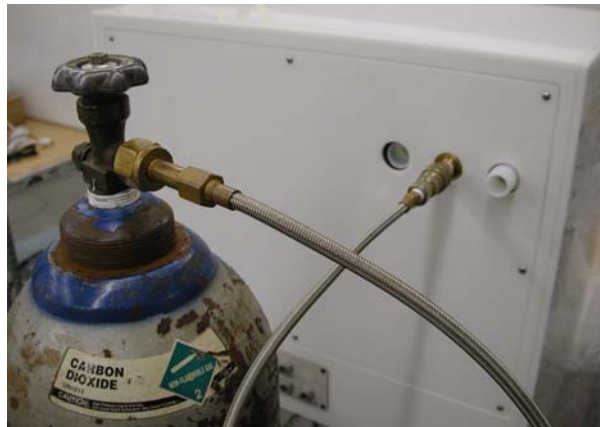
Figure 4.0-1: CO 2 cylinder hook up
