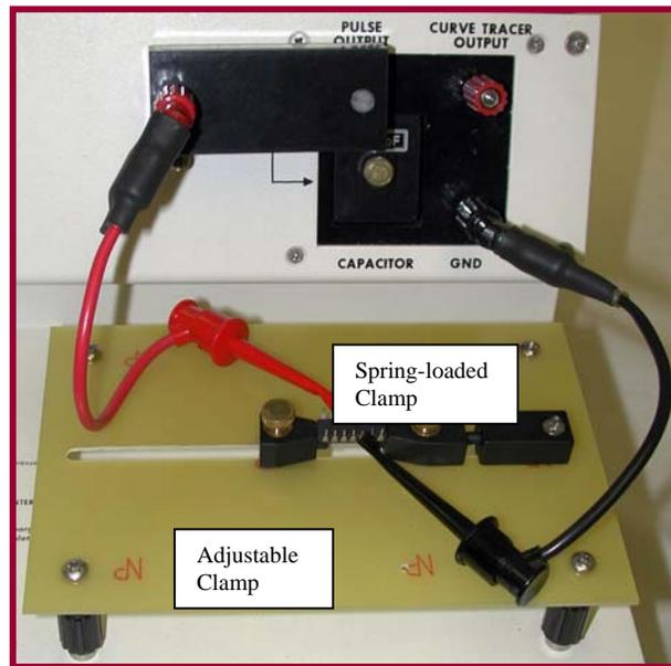
Figure 3.0-3: Universal Clamp Test Fixture (HBM)
