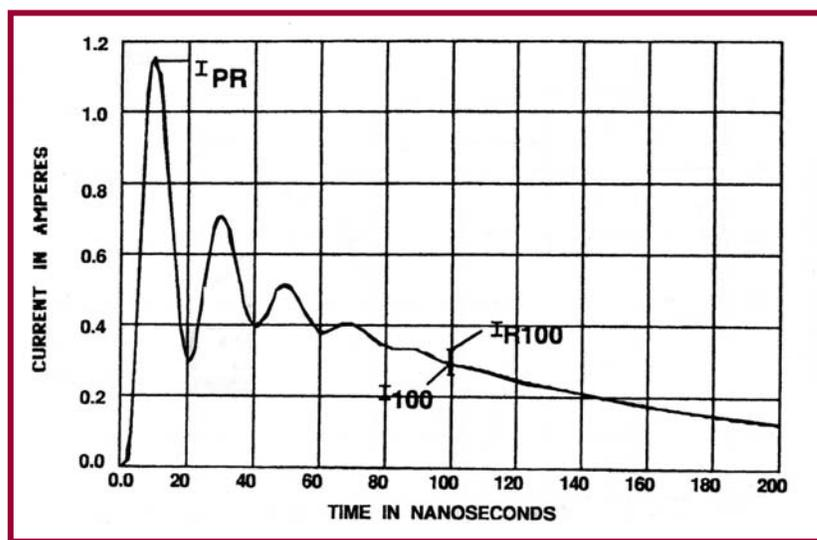
Figure 4.0-8: Current waveform through a 500 Ohm resistor to ground
