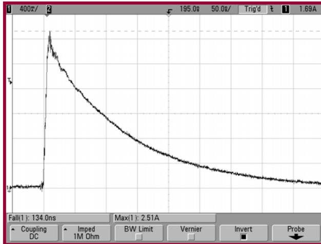
Figure 4.0-5: Discharge Pulse Fall Time Measurement at 4kV
