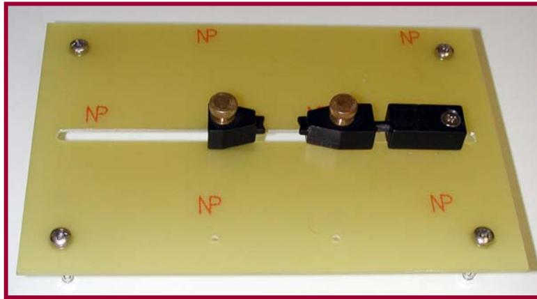
Figure 2.0-2: Standard universal DUT holding fixture
