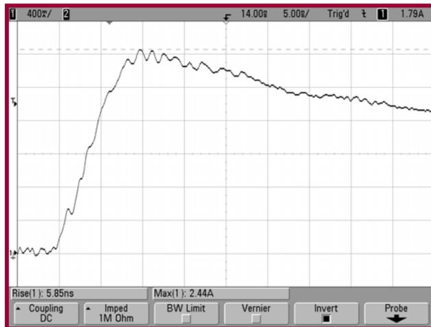
Figure 4.0-4: Rise Time and Ringing Waveform at 4kV
