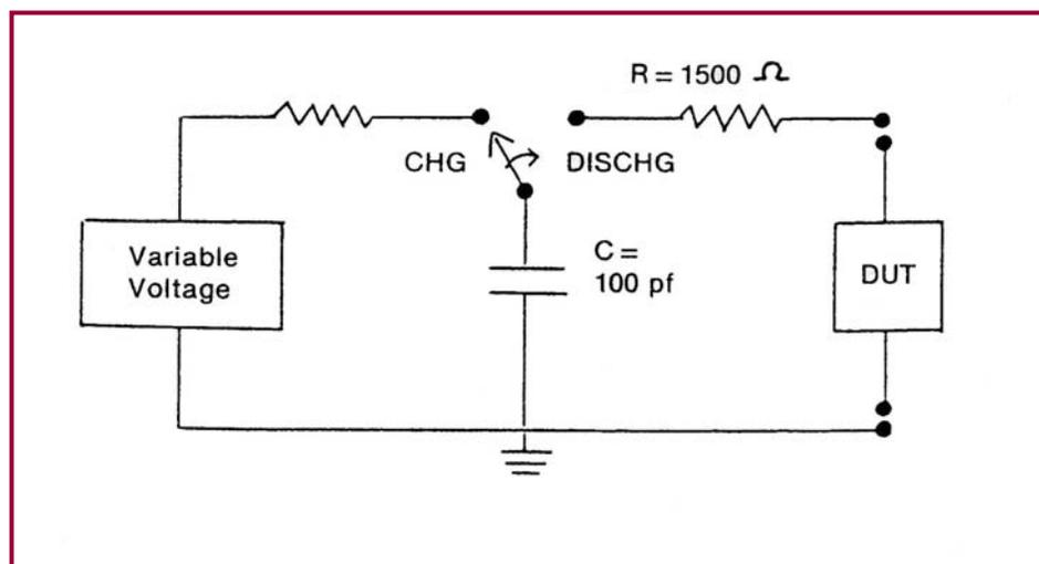
Figure 1.0-1: Basic Human Body Model equivalent circuit
