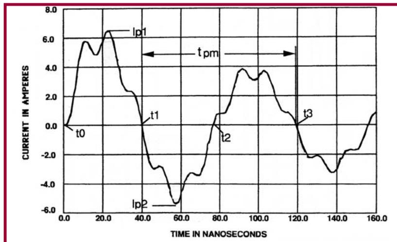
Figure 4.0-7: Current waveform through a short to ground
