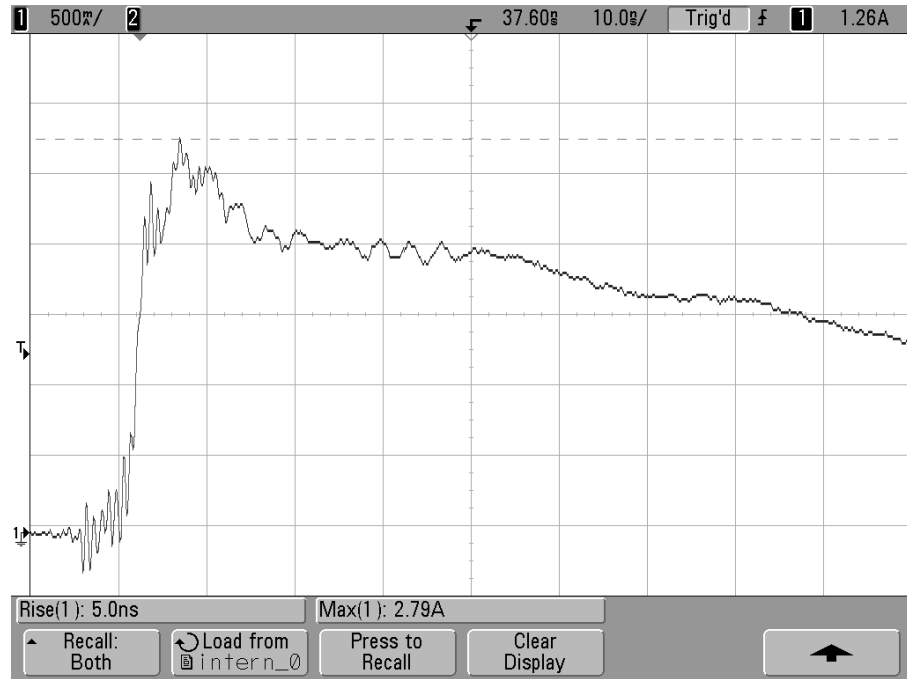
Figure 3.7-3: Typical HBM waveforms with Test Unit.
