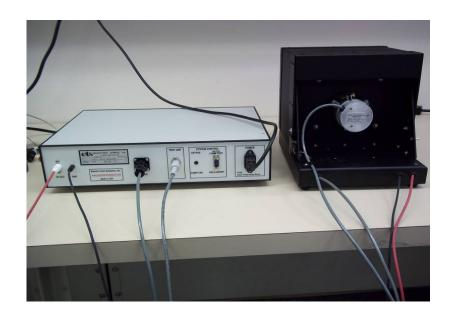
Step 2: Open Faraday cage cover and install STM-2 module as shown below
