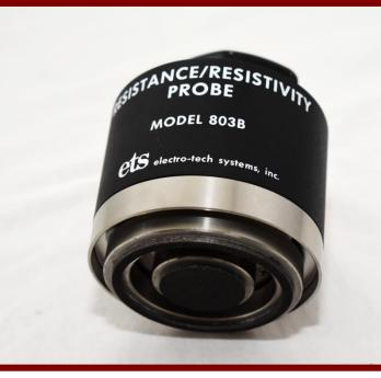
Evaluate your material's surface and volume resistance and resistivity characteristics. Electro-Tech Systems' 803 delivers critical insight on these metrics for planar surfaces. The electrodes are made from a conductive silicone for excellent probe-to-test-surface contact which allows measurements of 100 Ohms and greater to be made. The 803B comes complete with metal and acrylic test beds and is compatible the recommended Model 871 Wide Range Resistance Meter.
