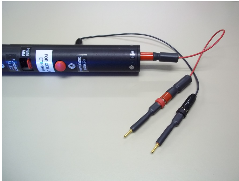
Figure 3.0-5: HBM test set up using external leads
