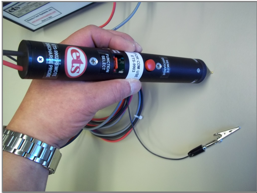
Figure 3.0-2: Holding Remote Probe
