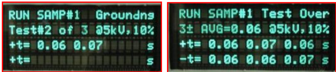
Figure 2.2-7: AUTO mode decay time measurement
