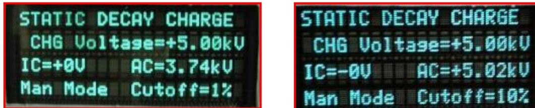
Figure 6-4: Sample with no IC and able to conduct charge
