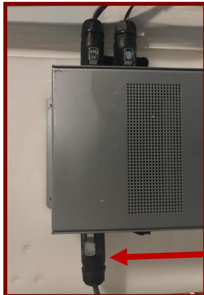
**Step 3.B. For a Dual Thermoelectric System (M 5477-500, M 5477-500-24), connect the 2<sup>nd</sup> thermoelectric.**
