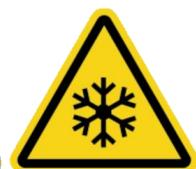
These symbols indicate extreme temperature which can cause burns or frostbite. Avoid contact with surface. Failure to follow precautions may result in moderate to severe injury.
